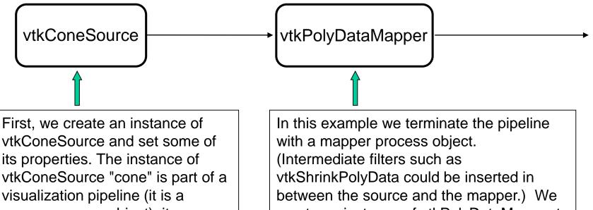
visualization pipeline (it is a source process object); it produces data (output type is vtkPolyData) which other filters may process.
