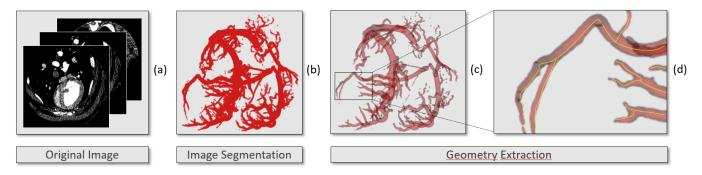
Figure 2: Example result of a student project. Original image (a) and its segmentation output (b). Based on the segmentation output isosurfaces (c) and centerlines (d) can be computed.
