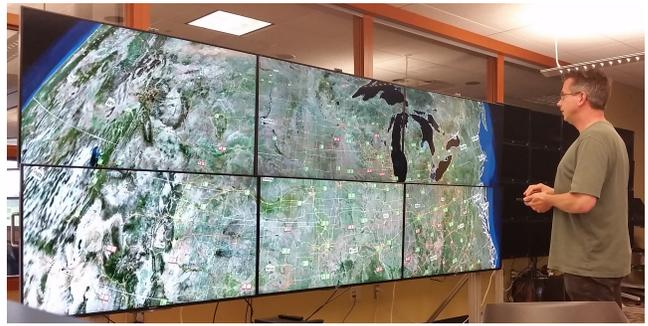
Figure 4: High-resolution tiled display system showing a GIS application based on OpenStreetMap.
