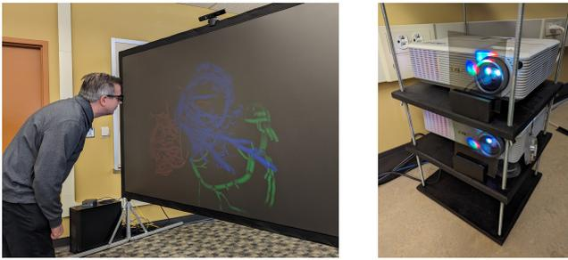
Figure 3: User exploring a vascular structure on a mobile projection-based VR display (left) and passive projector configuration for the display (right).
