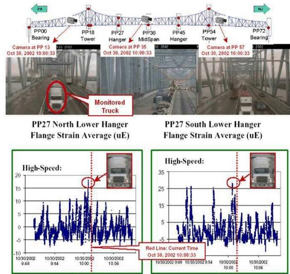
Figure 2. Bridge monitoring using cameras and conventional sensors (Commodore Barry Bridge, monitoring system by Aktan et al. [6]) (Schematic courtesy of E. Aktan).
