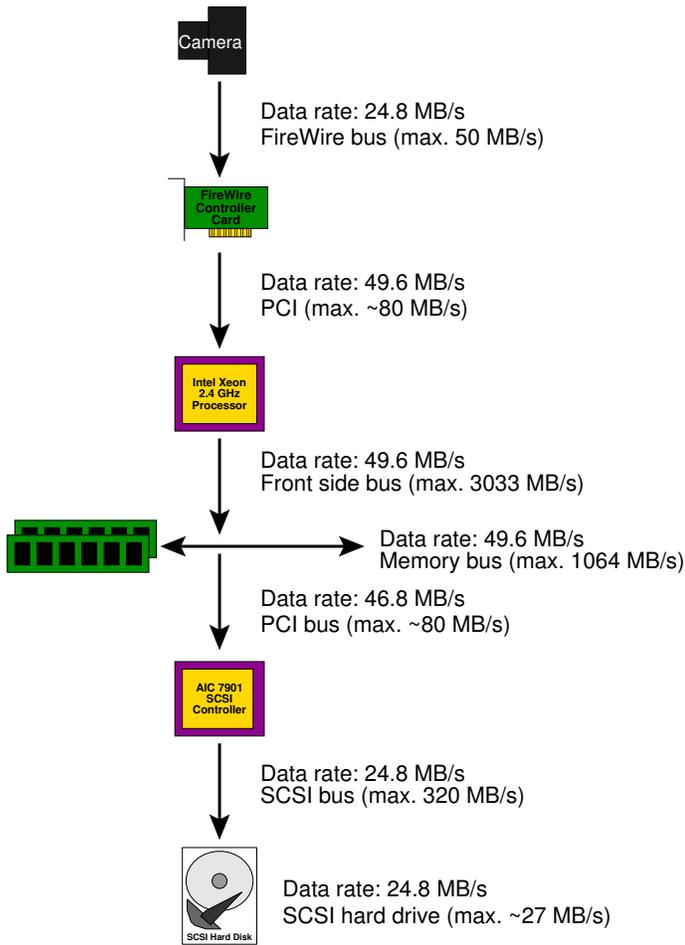
Figure 4. Data flow inside the computer system during capturing.
