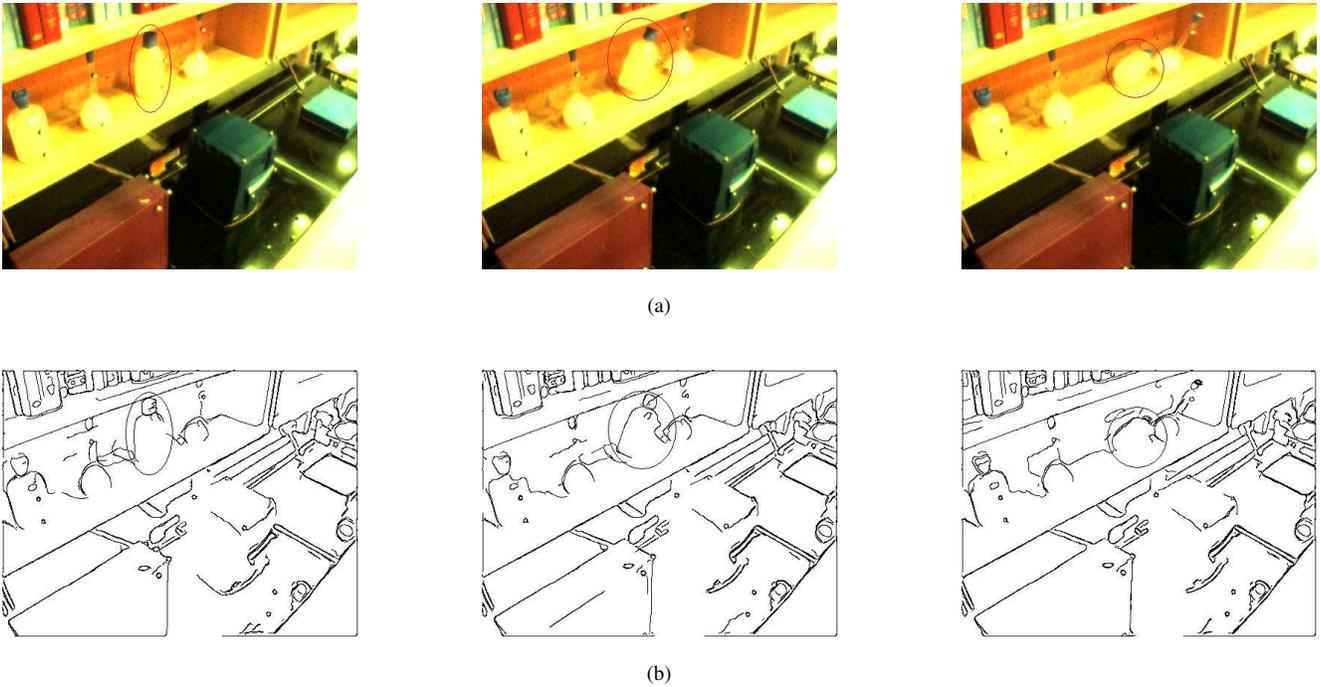
Figure 6. Chemicals observed by an optical sensor during a shake table experiment: (a) original images and (b) images with only edges identified. The tracked object is circled. Both, single shots of the video stream and detected edges are shown in subsequent order.
