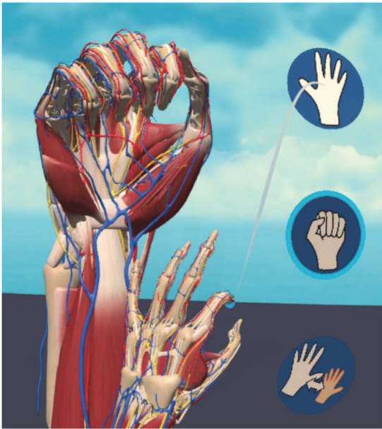
FIGURE 4. Immersive visualization offers many opportunities to explore complex medical data. In the educational tool pictured, users can explore anatomy of the hand in VR via live tracking of the user's hand in comparison to a bigger anatomical model. 12
