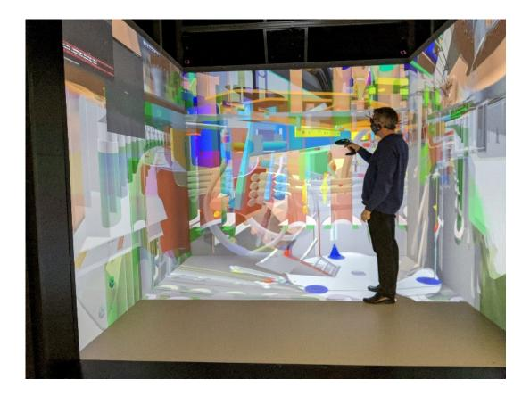
Figure 6. A user interactively exploring the design of a wind turbine in the Virtalis ActiveCube. The system enables to user look inside hidden objects or
