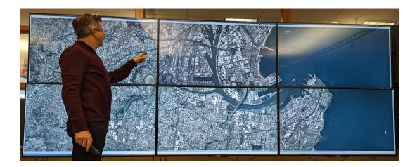
5 **Figure 4.** High-resolution tiled display system satellite imagery. The high resolution of the display can reproduce the fine details of the imagery when 6 exploring or discussing this type of data.
