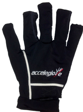
Figure 3. The AnthroTronix AcceleGlove used for collecting gesture data.
