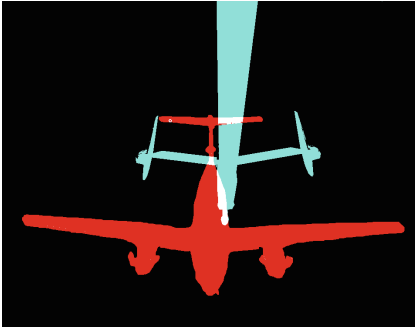
(a) From left camera POV, mask of boom (cyan) and plane (red), added creating overlapping pixels (white).
