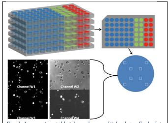
Fig. 1. An experimental batch can have multiple plates. Each plate has 384 wells. Each well is sampled at eight sites. Four images are captured at each site based on filters and dye frequencies.
