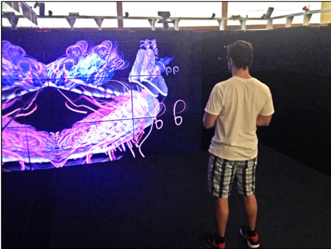
7 **Figure 5.** A user exploring a CFD data set describing the flow around a dragonfly's wings. The immersive and high-resolution capabilities of the DIVE system
