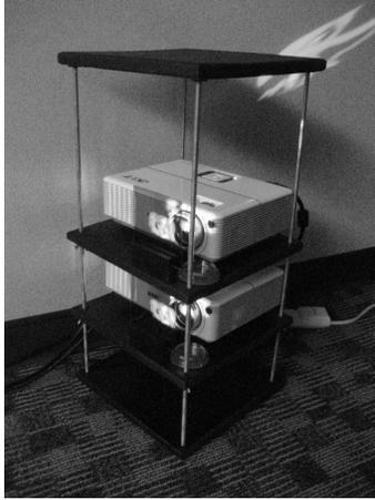
Figure 2. Set of projectors in a passive stereo configuration.
