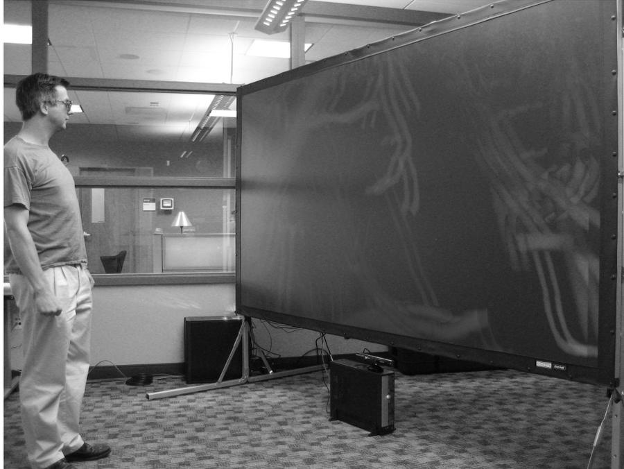
Figure 3. Tracked user in front of the passive projection screen with the tracking computer and the Kinect sensor on top underneath the screen.
