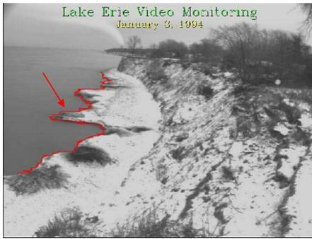
Figure 3. Growing ice at the shore highlighted by an edge detection algorithm (image courtesy of USGS [16]).
